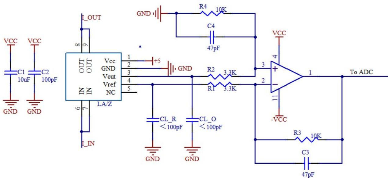
Typical application circuits for STB-LA current sensor. The magnification can be estimated as  $M = R4 / R2$  with the condition of  $R1 = R2$ , and  $R3 = R4$ . The magnification in the circuit above is around 3. The capacitive load of  $V_{out}$  and  $V_{ref}$  should not exceed 100pF to avoid oscillations.
